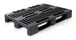
The ESD pallets out of electrically conductive plastic were especially designed for transporting sensitive electronic devices. They reliably prevent electrostatic charge and divert already existing charges.
