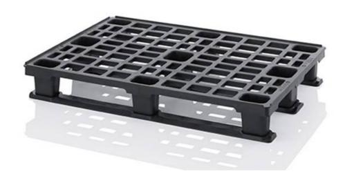
The ESD pallets out of electrically conductive plastic were especially designed for transporting sensitive electronic devices. They reliably prevent electrostatic charge and divert already existing charges. Special volume resistivity/surface resistivity: 10<sup>4</sup> < 10<sup>10</sup> Ohm.
